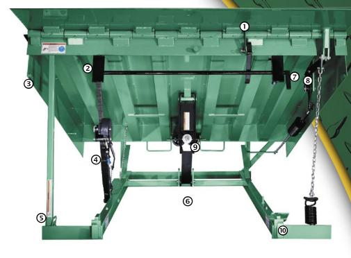
8 Hydra-Cam extends and holds lip at the top of its cycle. Lip remains yieldable throughout loading operation
