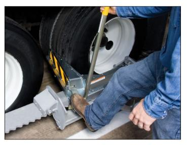
Once loading/unloading is complete, dock worker presses release button inside, alerting outside operator that it is safe to disengage wheel restraint. A simple press of the foot pedal disengages the restraining arm, rotating it back and away from the wheel.
