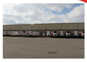
If overhead dock doors are not properly sealed, thousands of dollars of cold storage energy can be lost annually. To cap these losses, the Save-A-Lot facility installed the recently introduced VertiCool™ Door by TKO®, specifically designed for use with a vertical storing dock leveler to seal up the building envelope at thirteen dock positions along their cold storage shipping wall.
